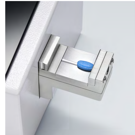
Quick-change tongue with groove for easy alignment of convex shapes
